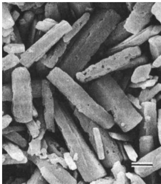
Figure 2 Scanning electron microscopic appearance of \text{Ga}_2\text{O}_3 particles. The bar represents 1 \mu\text{m} .
